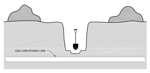
Dig a trench by hand across the full width of the excavation (perpendicular to or "across from" the line). If the line is not uncovered, mechanically excavate to one half the depth of the trench. Repeat this process until the line is exposed.
